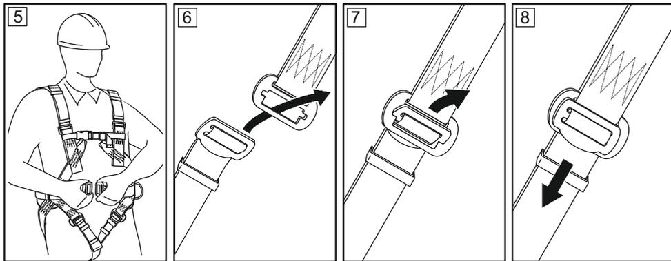
5 Adjusting the thigh straps and work positioning belt
