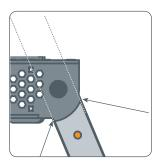
8. Install the Leg Restraint Straps (see section Leg Restraint Straps). Ensure the straps are adjusted so that all slack is removed. Where undulations or obstructions on the worksite surface prevent a clear path for the Leg Restraint straps the relevant straps must be adjusted such that the stability of the
