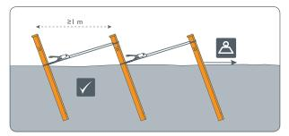
The stakes may be linked by 8 mm cord to EN 564 or by Lyon Ground Stake Linking Straps, which are tensioned between the stakes.
