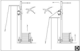
The device allows for operation only in direction shown in fig. A. It is forbidden to use the device in other directions as shown in fig. D. The DW100 trolley in combination with fall arresters and anchor lanyard AZ 800 for roof works have been tested for usage in the horizontal plane and fall beyond edge in accordance with Directive PPE 89/686/EEC + CNB/P/11.060.
