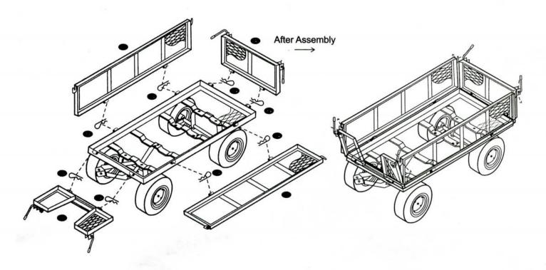
STEP 7: Latch the Fences in the upright position by closing the lock Handles
