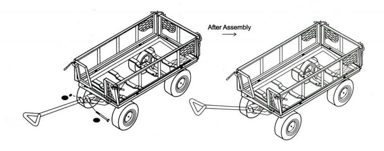
STEP 9: Make sure all bolts and nuts are securely tightened.
